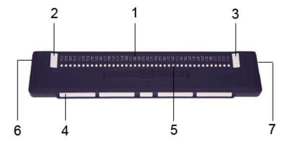
When the ALVA USB 640 Comfort is placed correctly in front of you, the Braille cells are located at the back of the flat surface, and the thumb keys are facing you.
